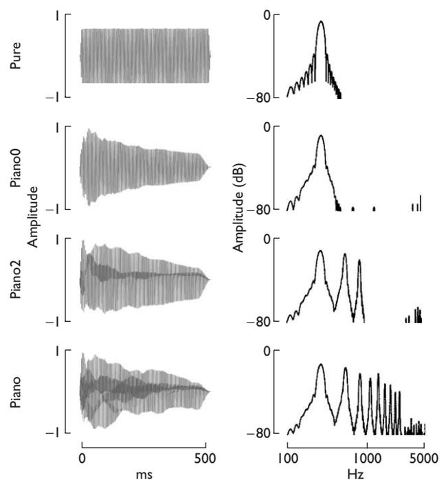
**Fig. 1** Time domain waveforms (left) and spectra (right) for the C4 stimuli. From bottom to top: piano tone (fundamental plus the first eight harmonics), piano2 tone (fundamental plus the first two harmonics contained in a piano envelope), piano0 tone (fundamental contained in a piano envelope), and a pure tone with only the fundamental.
